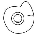
WHEN CAM IS CORRECTLY INSTALLED, THE HUMP IS AT THE TOP.
